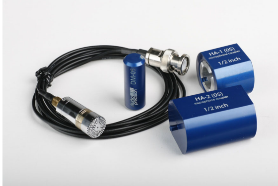
Measurement microphone, dummy mic, HA-1 and HA-2 couplers.
