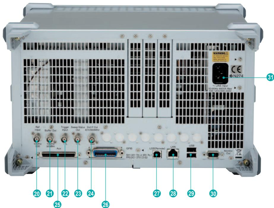
**20 Ref Input connector (reference frequency signal input connector):** Inputs an external reference frequency signal (10 MHz/13 MHz). It is used for inputting reference frequency signals with accuracy higher than that of those inside the MS269xA, or for synchronizing the frequency of the MS269xA to that of another device.
