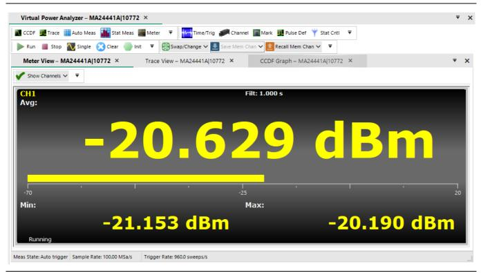
Figure 4-29. The Meter View Measurement Display Window
