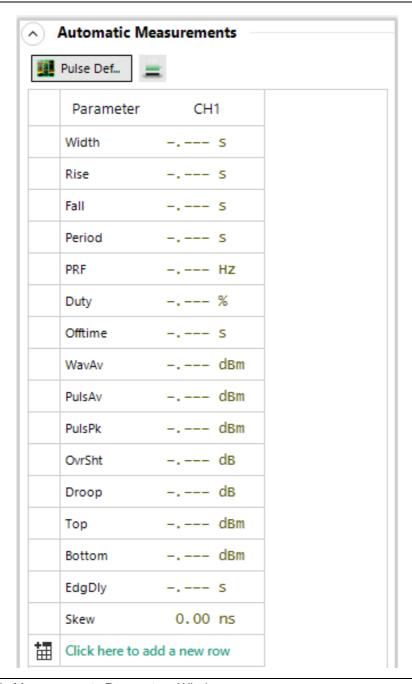
Figure 4-20. Automatic Measurements Parameters Window
