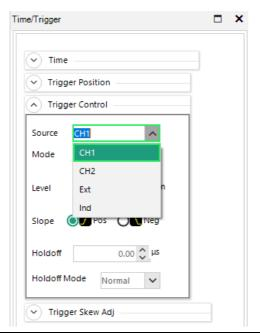
Figure 4-36. Trigger Source Selection Dialog for Two Sensors
