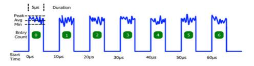
Figure 4-40. Sample Burst Signal Showing Buffer Entry Elements
