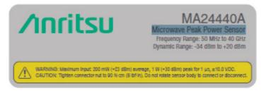
Figure 3-4. Information Labels on the MA244xxA Peak Power Sensor
