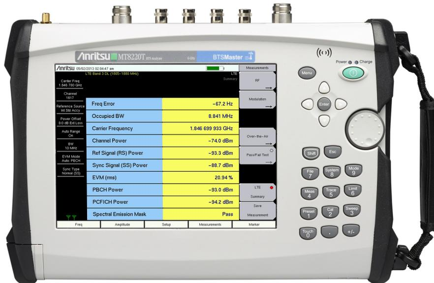
BTS Master™ MT8220T Base Station Analyzer featuring Vector Signal Generator
