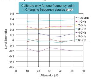
The absolute amplitude accuracy specifications of other spectrum analyzers excludes:
